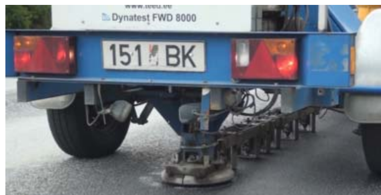
Figure 3-4: Falling Weight Deflectometer (Engtec, 2018)
