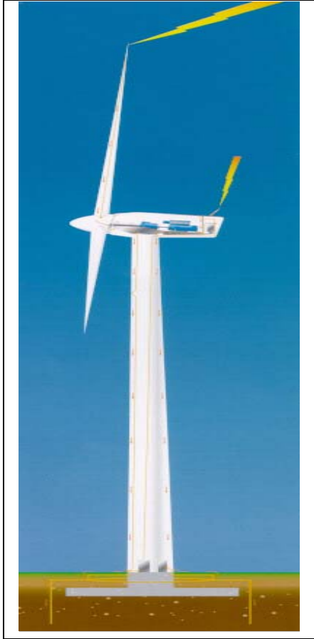
Exhibit 1.5-10 Typical WTG Lightning Diversion Paths
