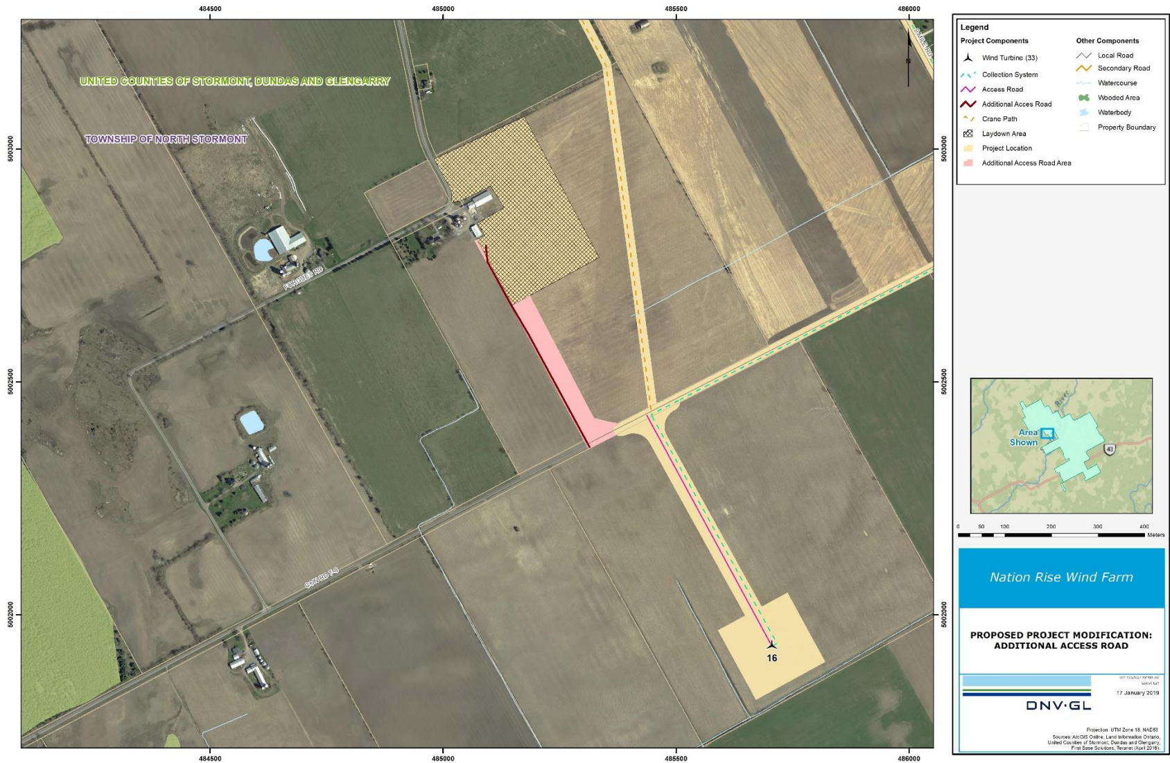
Figure 3-2: Propose Layout Modification for the Additional Access Road to the Central Laydown Yard
