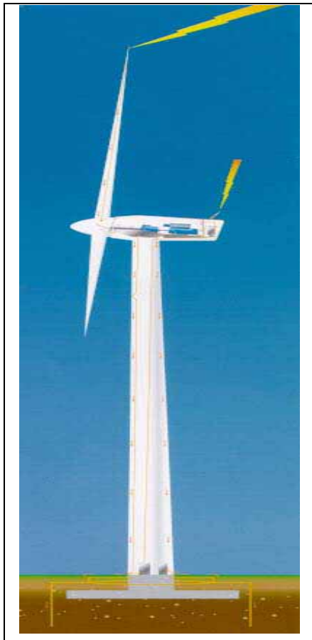
Exhibit 1.5-10 Typical WTG Lightning Diversion Paths
